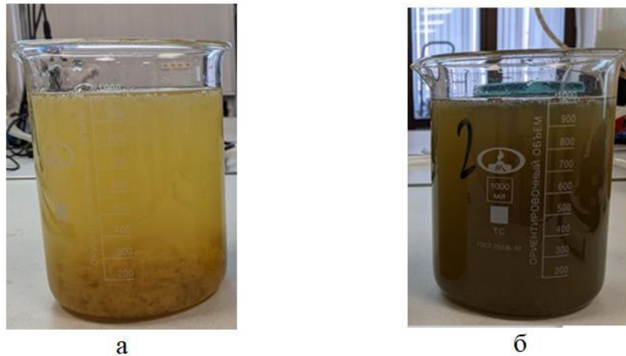
Figure 3. Model wastewater after coagulation, neutralization and flocculation: enlargement of flocs and separation of the sediment phase. Adapted from the experimental source.
