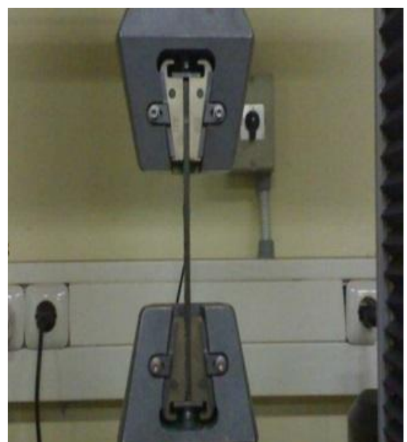
Figure 11. Universal testing machine and specimen held in grips
