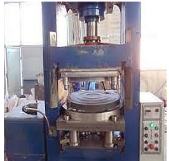
Figure 16. The process of pressurizing with a hydraulic press
