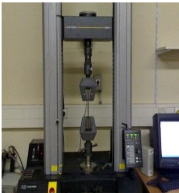
Figure 11. Universal testing machine and specimen held in grips
