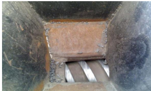
Figure 7. The rotator of the mixing machine
