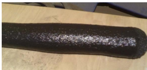
Figure 8. Recycled plastic paste after exiting the extruder machine
