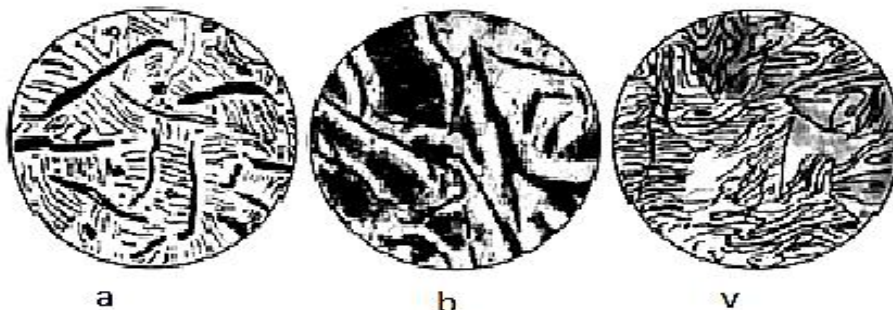
Figure 2. Microstructures of cast gray cast irons: a - ferrite-graphite; b - ferrite-pearlite; c - pearlite
