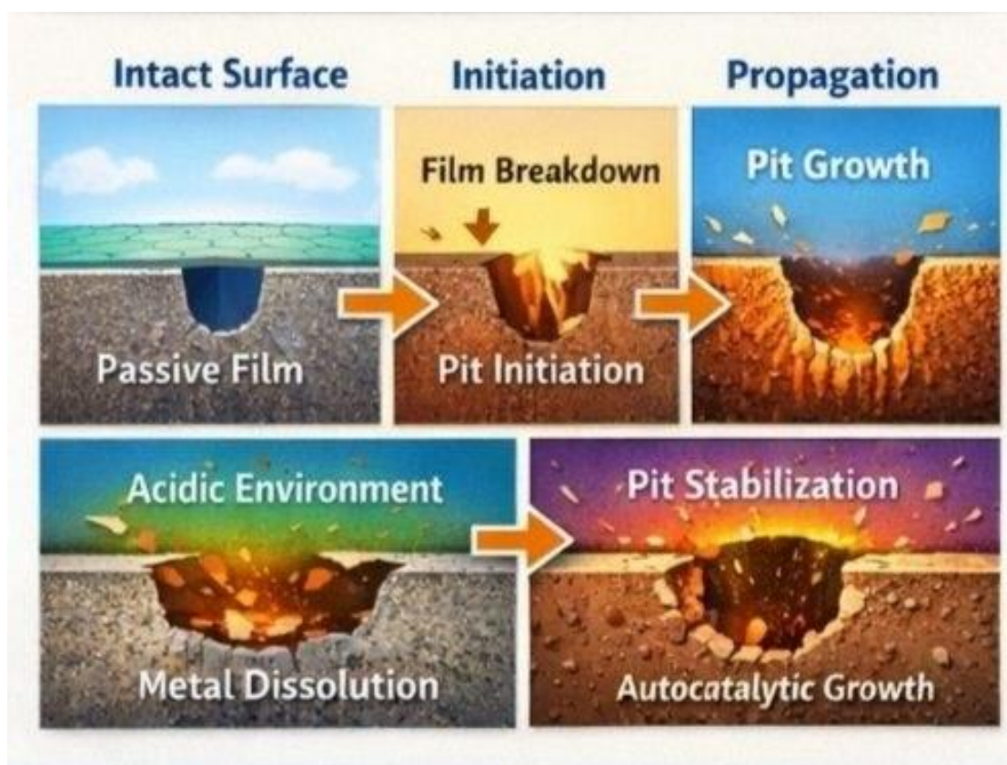
Figure 1. Schematic of pitting corrosion mechanism.
