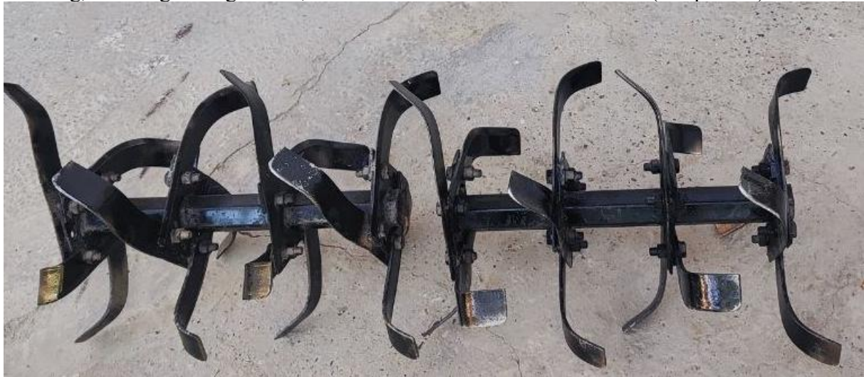
3.3–picture. Soil-softening milling machine
