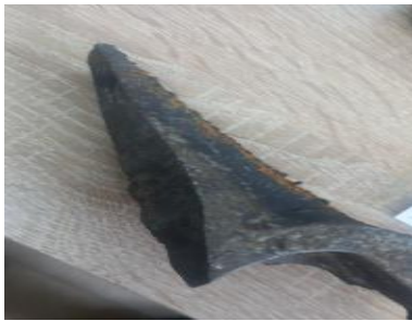
Figure 3. Carbide oxide composite material obtained in laboratory conditions.
