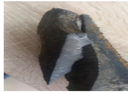
Figure 3. Carbide oxide composite material obtained in laboratory conditions.
