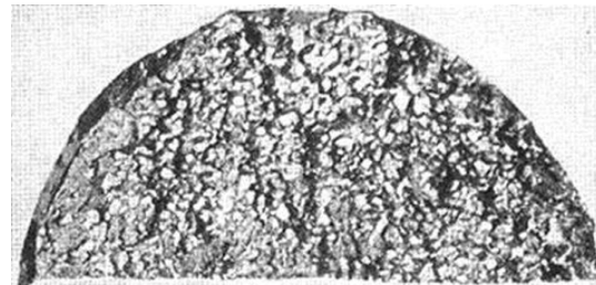
Figure 3. Viscous fracture Fig. 4. Intercrystalline brittle fracturing. increased by 3times
