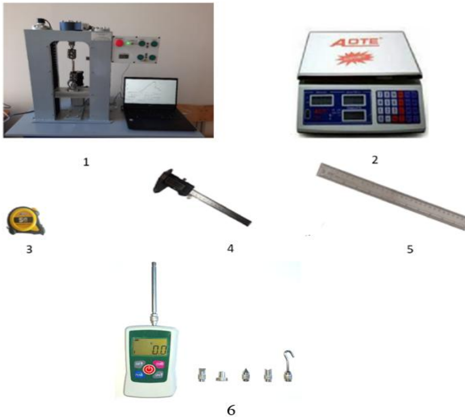
1 - installation of UEIM20300; 2 - scales; 3 - tape measure; 4 - calipers; 5 - ruler; 6 - dynamometer DIGITAL FORCE GAUGE AMF-500
